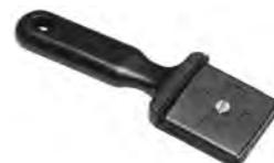
The Stabi-Pipes are finished with an aluminium coating on their outer surface. This aluminium coating has to be scraped off within the welding section before welding the pipe. Each peeling tool is designed for two individual pipe diameters. The peeling tools for diameters from 50 mm on have turning handles.
